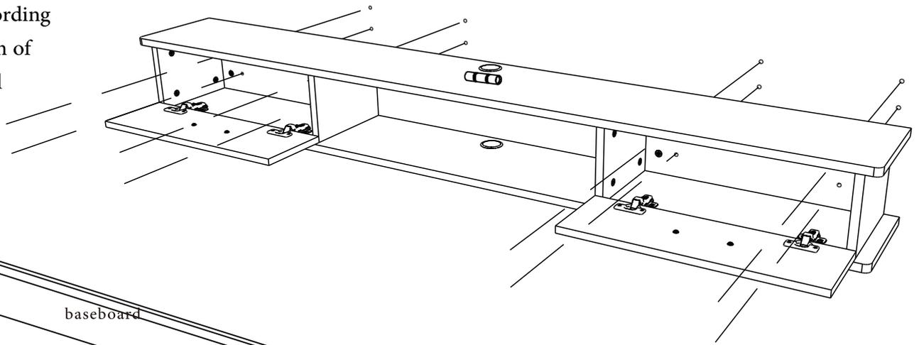
Drill 8mm holes on the wall according to the pre-holes
