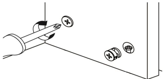
put the fasteners into the holes and screw it with a screwdriver
