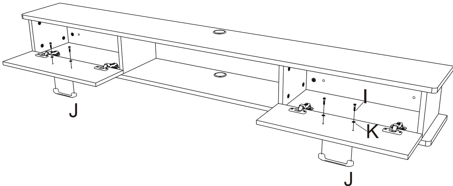
Locate the hole on the wall of the furniture according to the position of the spirit level
